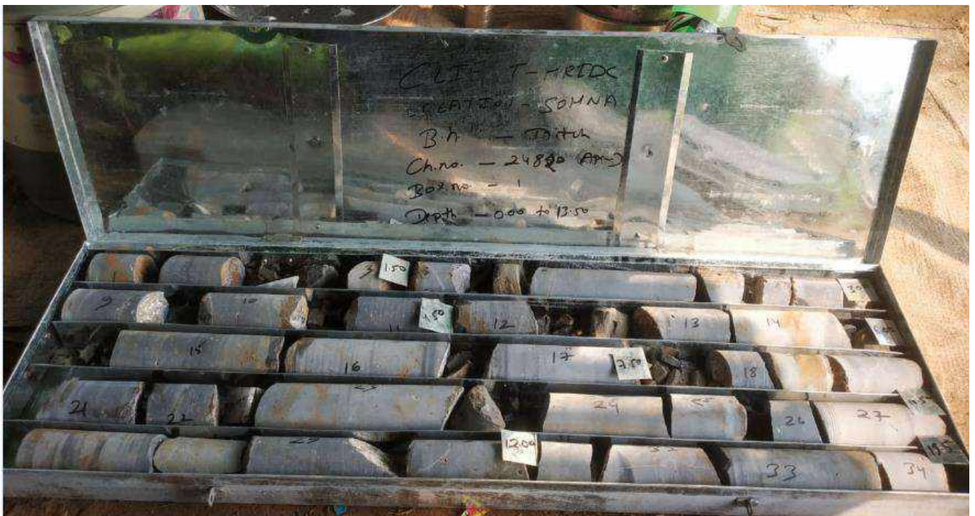
BH 15(A) Box 1. (Depth 0-13.5m)
