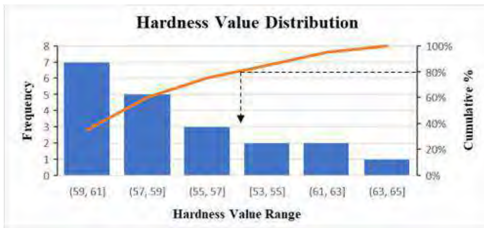
Figure 4.14: Pareto Chart showing recommended Hardness value for the rock mass within 2D depth.
