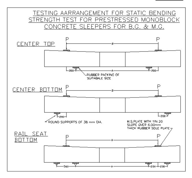
Note:- The testing arrangement is for guidance purpose only. Testing shall be conducted as per test loads mentioned in the relevant RDSO's drawings of PSC sleepers. The dimensions A & B mentioned in above testing arrangement shall be referred from relevant RDSO's drawing of PSC sleepers.
