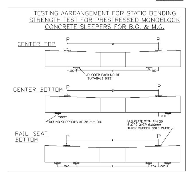
Note:- The testing arrangement is for guidance purpose only. Testing shall be conducted as per test loads mentioned in the relevant RDSO's drawings of PSC sleepers. The dimensions A & B mentioned in above testing arrangement shall be referred from relevant RDSO's drawing of PSC sleepers.
